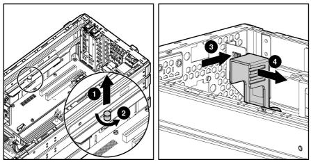
Figure 1-11: Unlocking the system board tray
